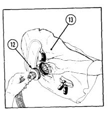
r. Screw cap (14) onto hose inlet adapter (12). Hand tighten.
