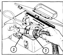
g. Read pressure gage (8). Reading must be at least 2.0 in. of water (3.0 cfm). If pressure is met, go to step o. If pressure is less, note reading and go to step h.
