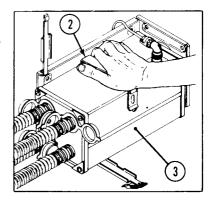
y. If air purifier (3) was pulled out, put air purifier back into mounting bracket (13) and fasten catch (12).
