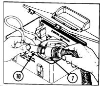
z. Read pressure gage (15). Reading must be at least 2.0 in. of water (3.0 cfm). If pressure is less, note reading.
